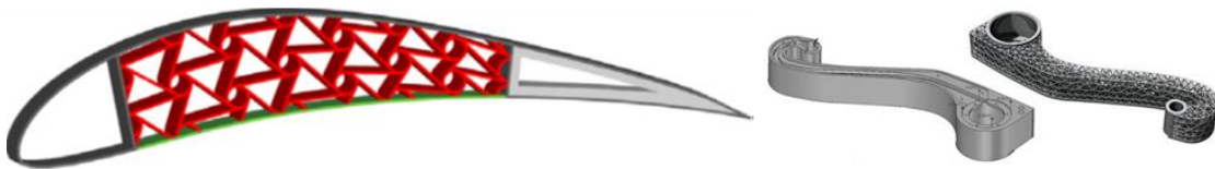
Fig.1: auxetic actuated wingbox (left) and AM optimized parts (Airbus, right)
